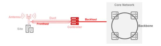
Figure 1. Mobile network and the scope of mobile backhaul
